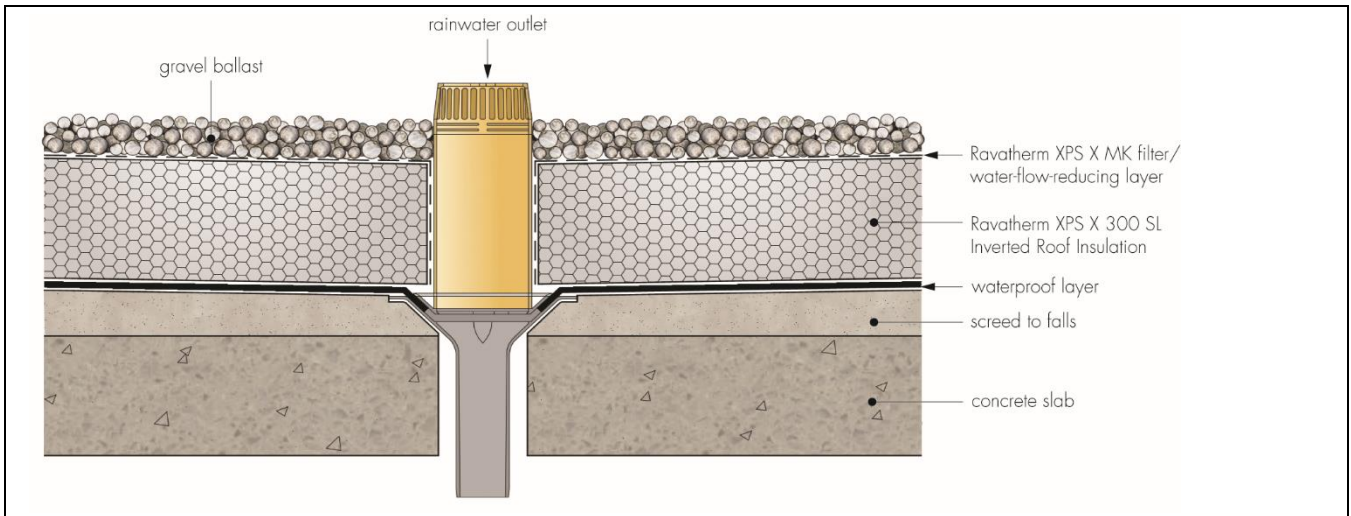
Figure 3 Water outlet detail — gravel finish
